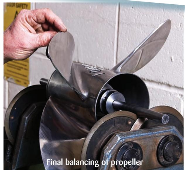
Final balancing of propeller
