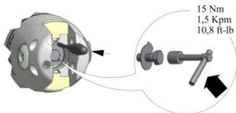
**3** Again using a straight screw driver: Bend side of tab washer up over hex on the shaft nut locking screw (6).
