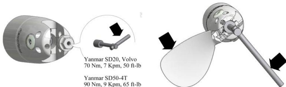
**2** Slide tab washer (5) on to shaft nut locking screw (6); screw in through hole in the shaft nut into end of shaft and tighten firmly; If using torque wrench tighten to about 15 Nm;
