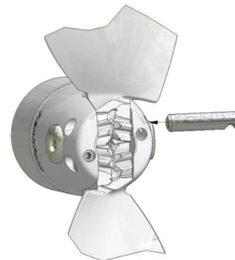
**7** Insert last pivot pin locking screw (9); turn it to engage a couple of threads; It will be tightened later in step 8;
