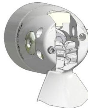
**6** Align last blade (7) in hub jaw and insert pivot pin (8) with the notch in pin aligned with the hole for the pivot pin locking screw; Move blade slightly to ease operation;
